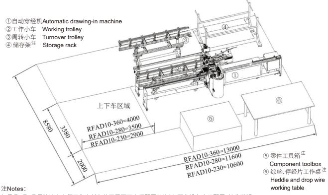
标号④、⑤、⑥是建议客户便于生产任务的开展而可自行配置的物料,而非设备出厂配置,特此说明。 The material of ④、⑤、⑥ shall be prepared by customer; not supplied along with machines.
